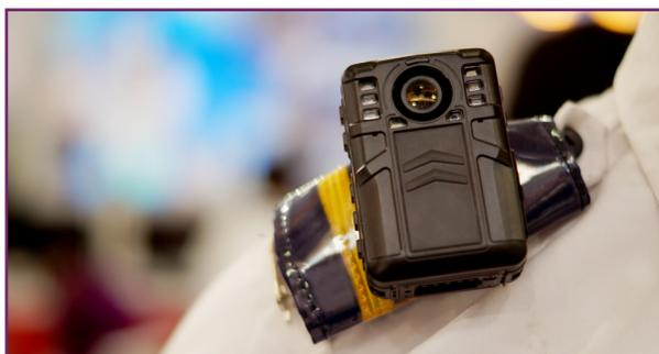
pocket-sized battery pack which may ensure recording capability during an entire shift. Alternatively, they may be powered by a rechargeable battery with a range of battery life depending on the chosen camera and battery. When recording, the camera captures a wide-angle, full-color view of objects and persons directly in front of an officer.
